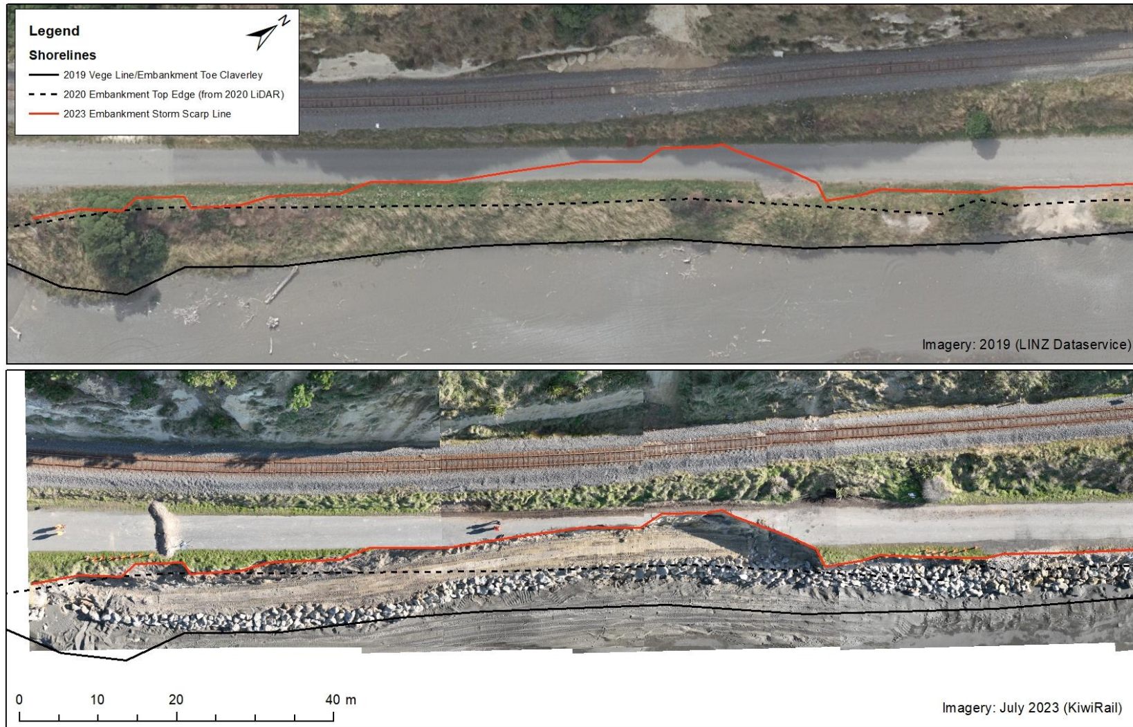
Figure 3.3: Comparison of shoreline reference positions and underlying aerial imagery from 2019 and post-slip in July 2023
